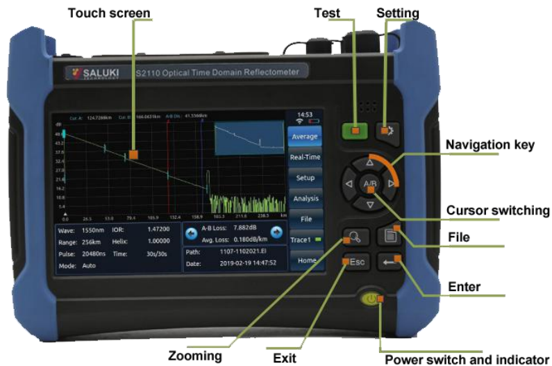
Fig.1-1 Front panel of the S2110P optical time domain Reflectometer
