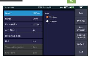
**IOR:** provided by optical cable or fiber manufacturer. It is the key parameter for calculating the distance, and can not be set arbitrarily.
