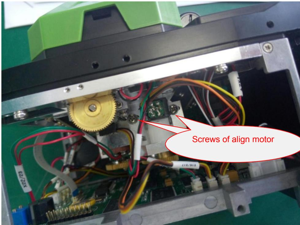
Fig.8 Align motor
