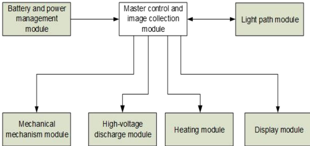
Fig.2 Block diagram of whole machine
