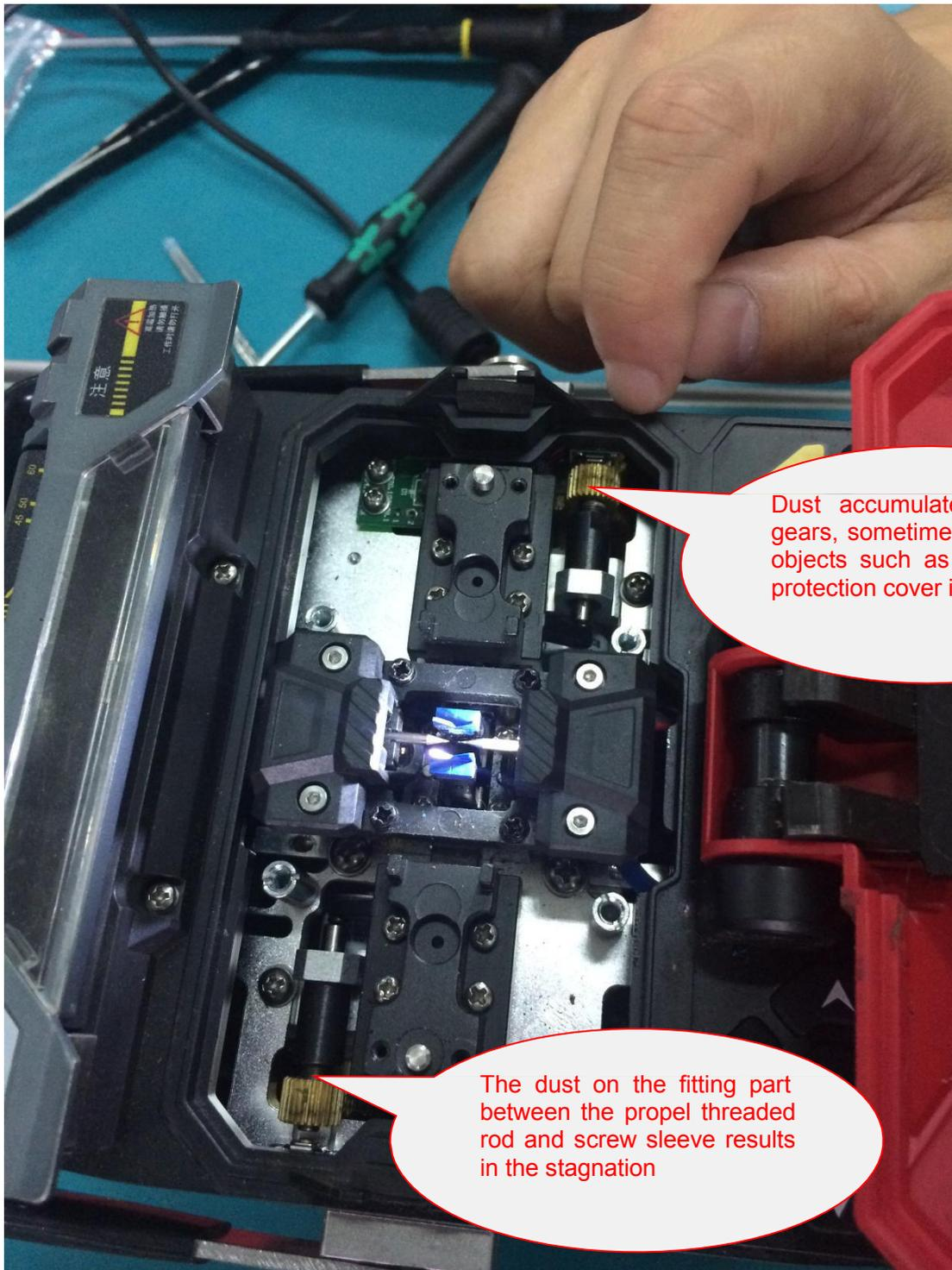
Fig.5 Cleaning of foreign objects between motor gears
