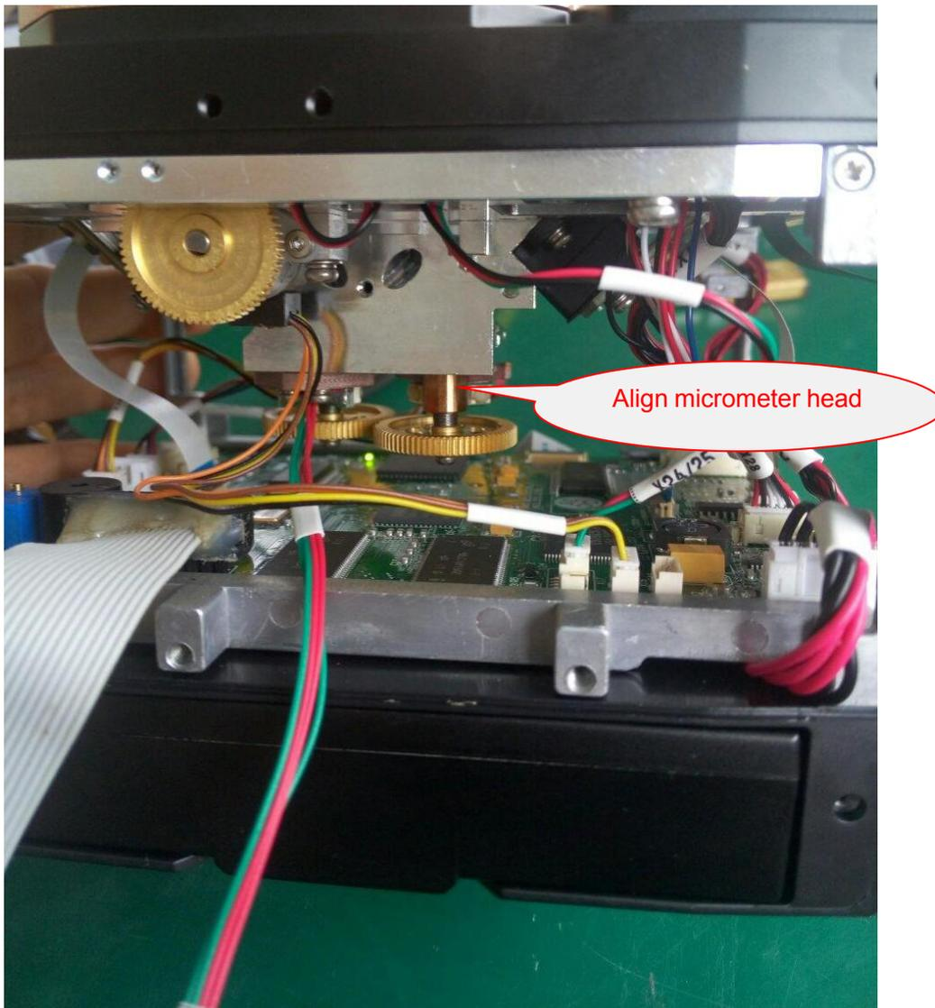
Fig.9 Align micrometer head
