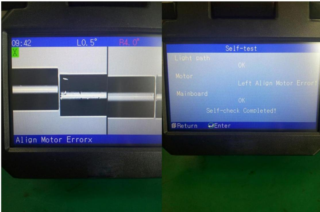
Fig.7 Jam of align motor
