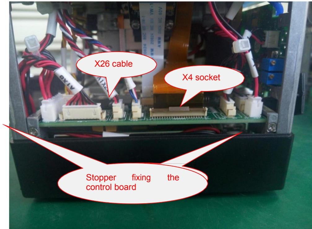
Fig.19 Stopper of main control panel
