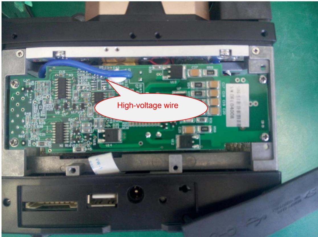
Fig.17 High-voltage board
