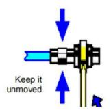
Fig. 2.5 Completion of final connection with a torque wrench
