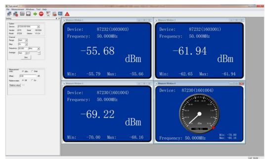
Fig. 3.6 Measurement window connected with multiple USB CW power sensors
