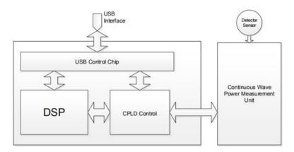
Fig.5.1 Block diagram of USB continuous wave power sensor
