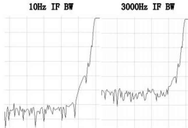
Fig.12 Influence on measure result from intermediate-frequency bandwidth
