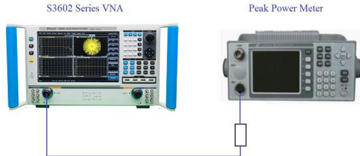
Fig. 11.14 Block Diagram of Test of Pulse Modulation Rising/Falling Time Indicators
