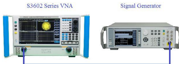
Fig. 11.6 Block Diagram of 1dB Compression Level Test of Port
