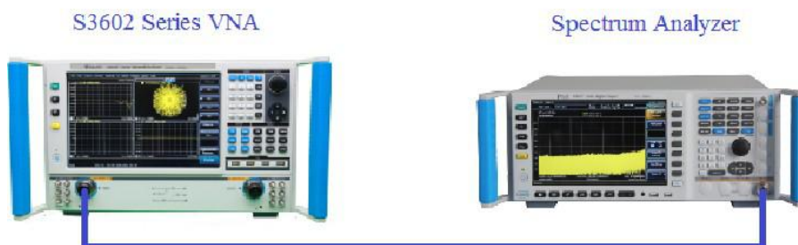
Fig. 11.5 Block Diagram of Pulse Modulation Switching Ratio Test
