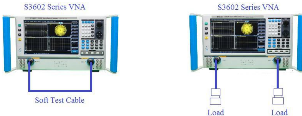
Fig. 11.8 Block Diagram I of Dynamic Range Calibration Test of System
