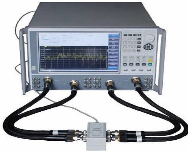
Fig. 7.29 Connection of Four-port Network Analyzer and Electronic Calibration Kit
