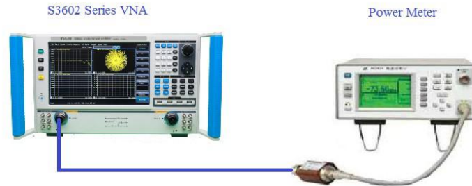
Fig. 11.4 Block Diagram of Port Output Power Test
