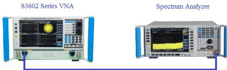
Fig. 11.2 Block Diagram of Frequency Resolution Test
