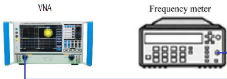
Fig.11.1 Block Diagram of Frequency Accuracy Test
