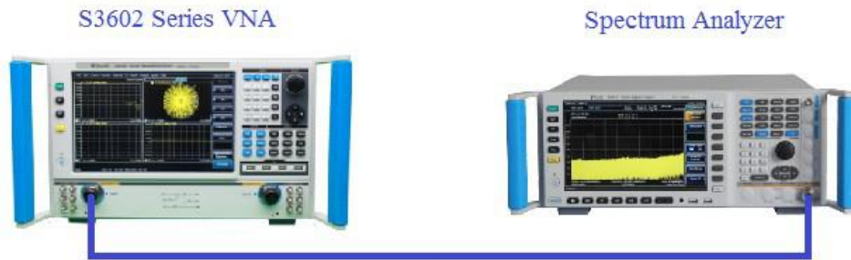
Fig. 11.3 Block Diagram of Test of Harmonic/Non-harmonic Suppression Test
