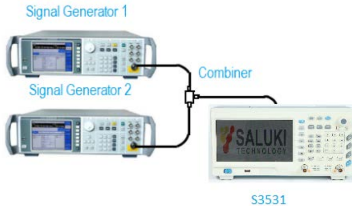
Fig 5-2: Equipment Connection for 2 signal capture
