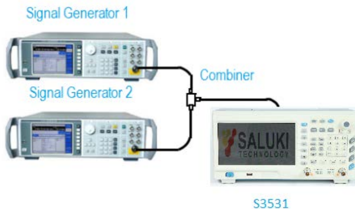
Fig 5-14: TOI Distortion Measurement Connection
