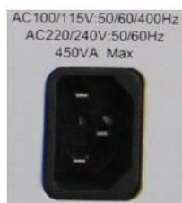
110 V/220 V self-adaptive AC power module
