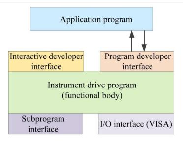
Fig. 2.7 Instrument Driver Structure Model
