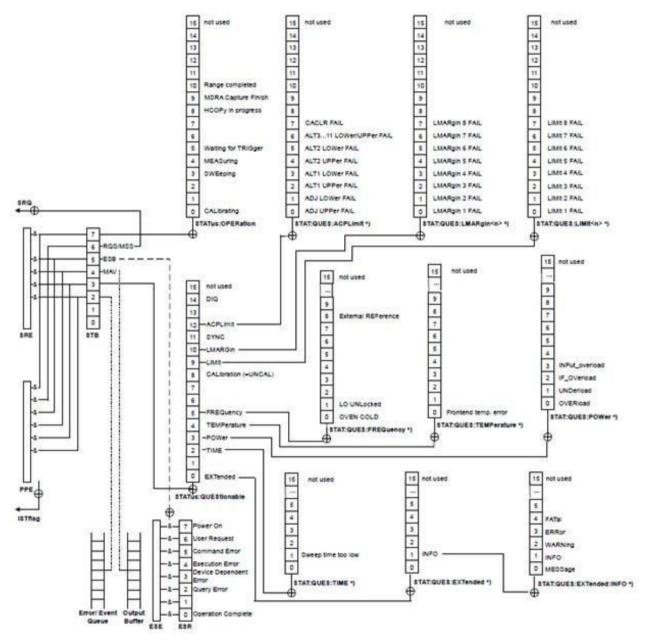
Fig. 2.3 Hierarchical Structure of Status Register
