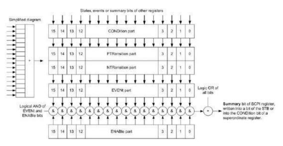
Fig. 2.4 Structure of Status Register
