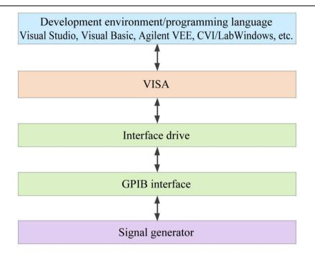
Fig. 4.1 Programming Software and Hardware Layer
