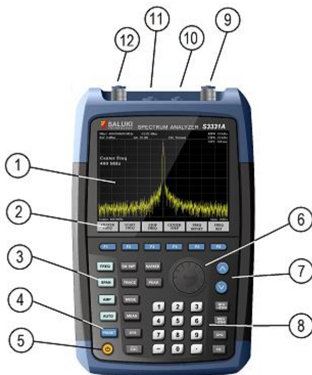
Figure 3-1 Front Panel of S3331 handheld spectrum analyzer
