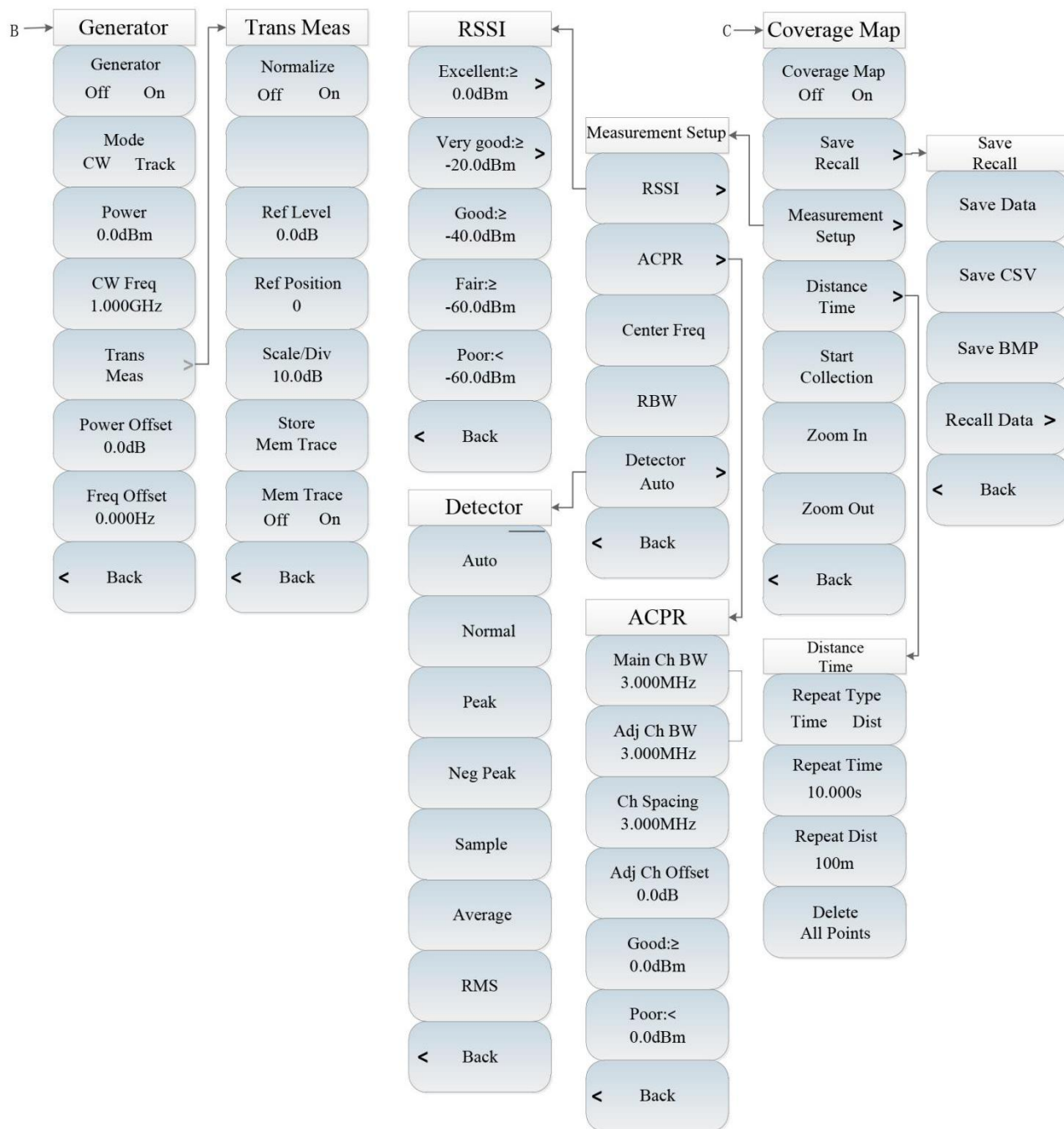
Fig. 4-33 Overall Block Diagram of Spectrum Analysis Menu (continued)
