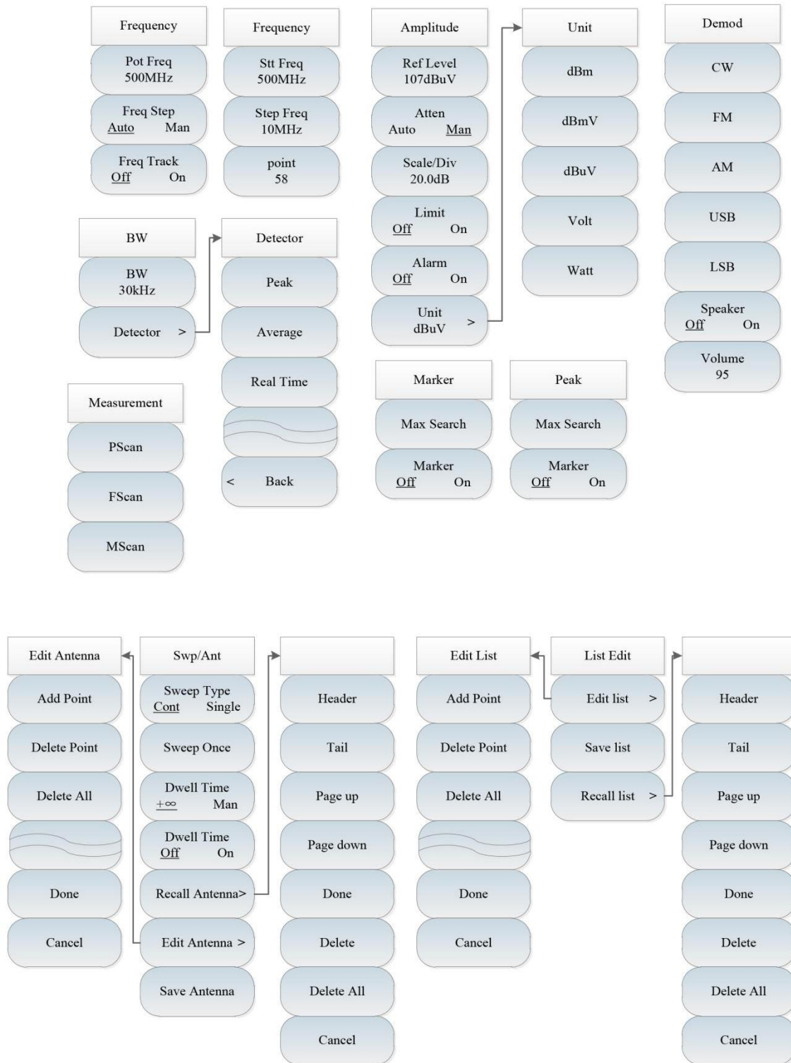
Fig. 9-4 Overall Block Diagram of Field Strength Menu
