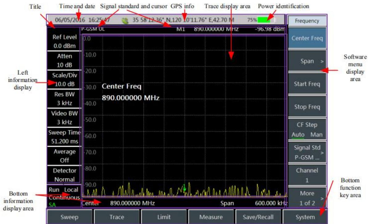
Fig.2.2 Operation interface of S3302 series spectrum analyzer
