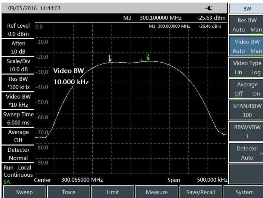
Fig. 3.13 Distinguishable two signals with same amplitude
