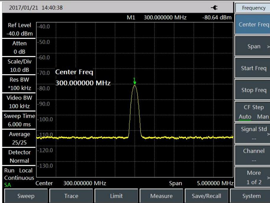
Fig. 3.10 Measuring Small Signals by Using Track Average
