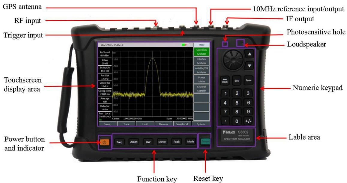
Fig.2.1 Front panel of S3302 series spectrum analyzer
