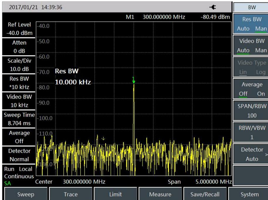
Fig. 3.9 Measuring Small Signals by Reducing Resolution Bandwidth
