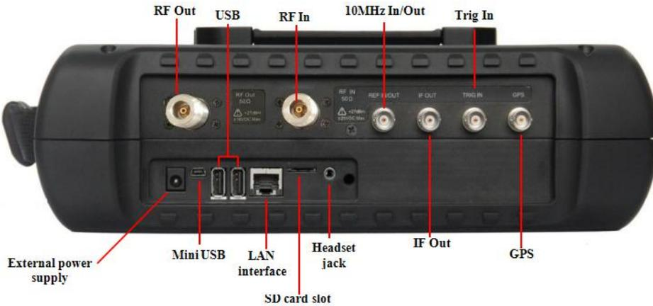
Fig.2.3 Top Panel of S3302 Series Spectrum Analyzer
