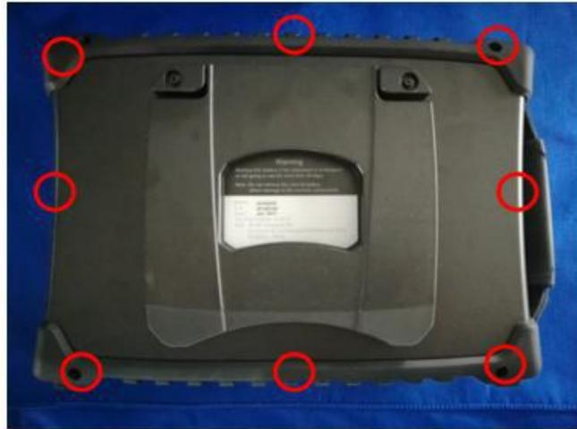
Fig.4 Removal of 6 fixing screws
