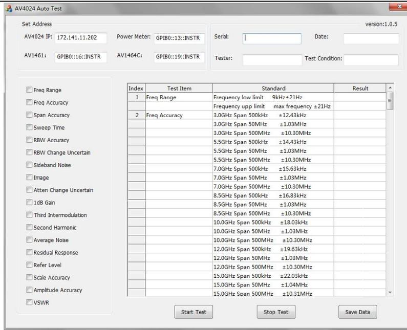
Fig.17 Interface of the automatic test of indexes
