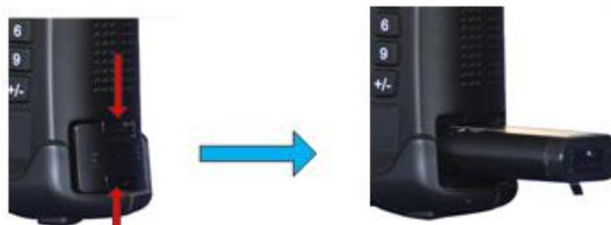
Fig.3 Removal of battery
