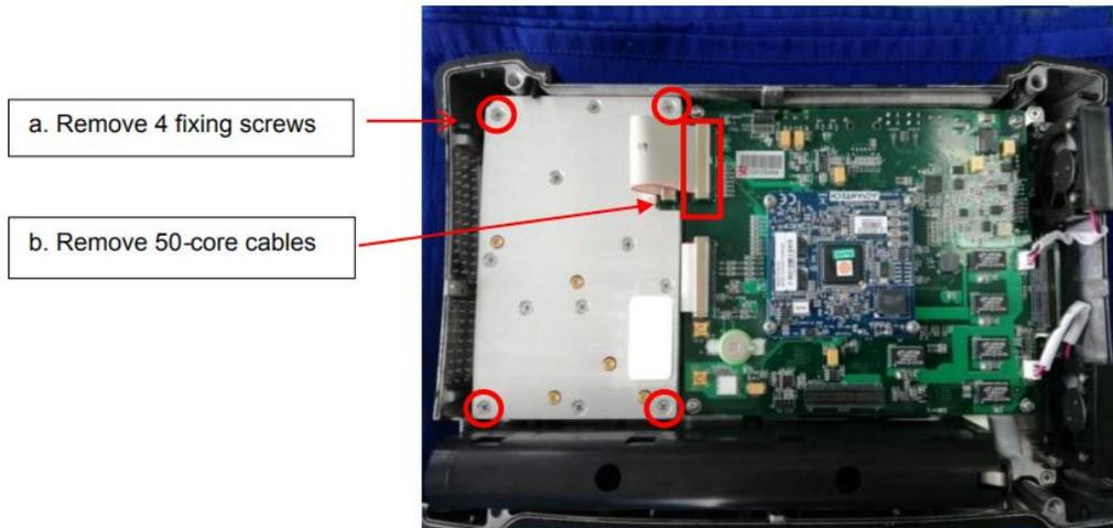
Fig.8 Removal of the IF channel plate
