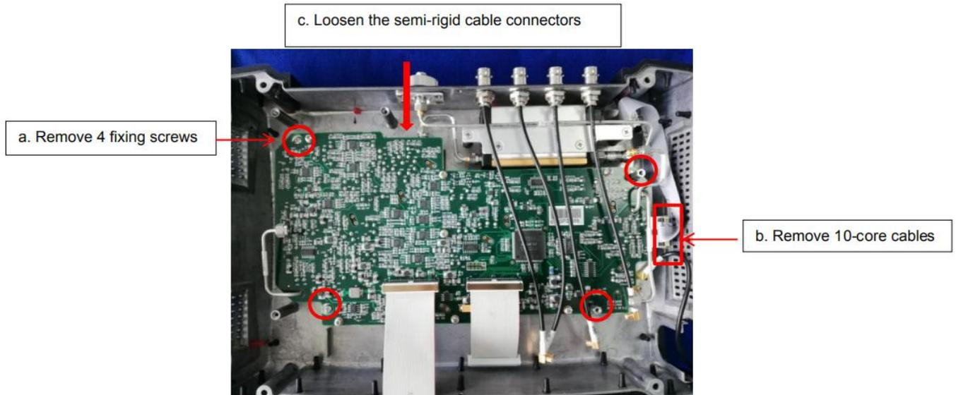
Fig.7 Removal of the microwave/millimeter-wave frequency conversion module
