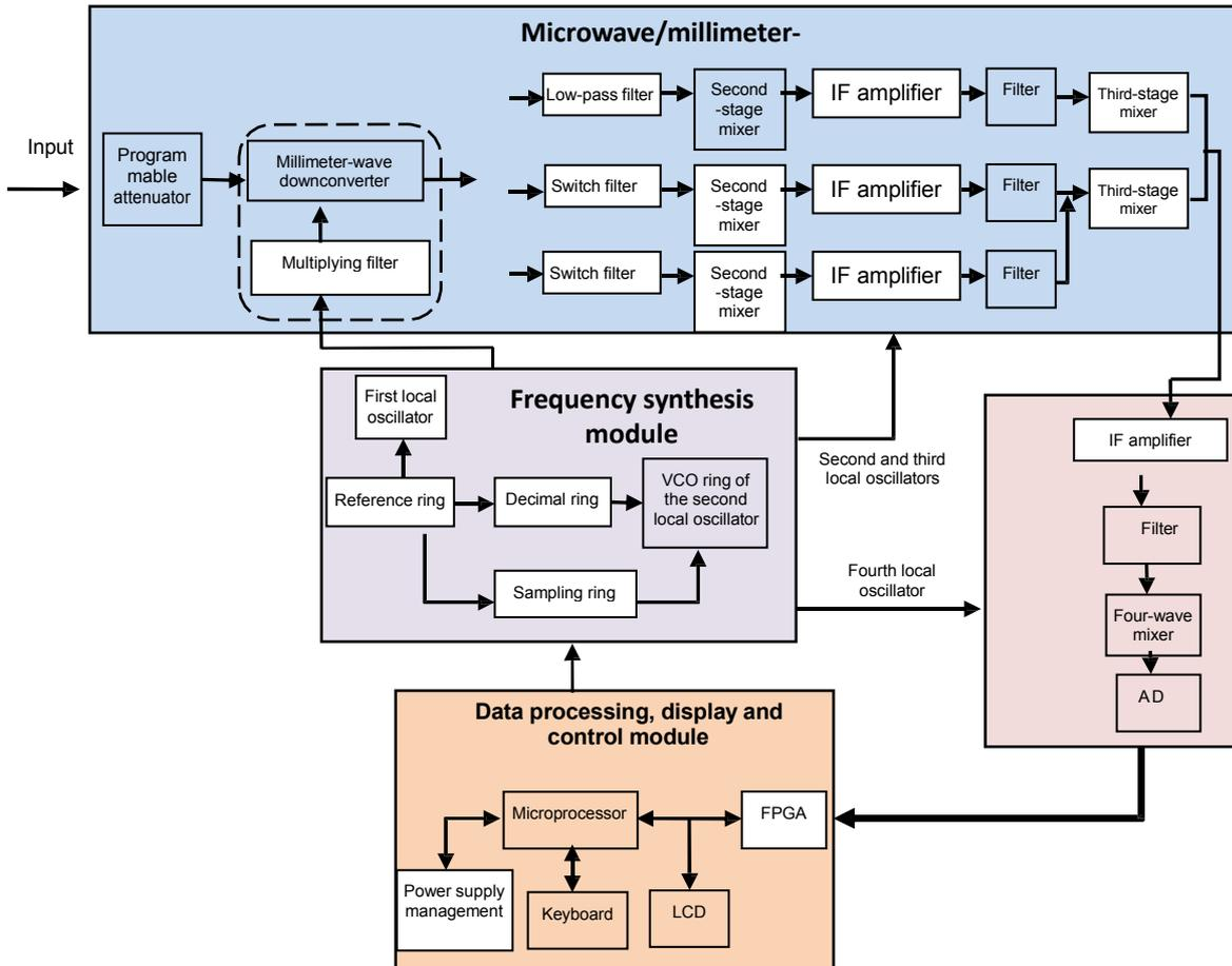
Fig.1 Diagram of Hardware of the Main Unit
